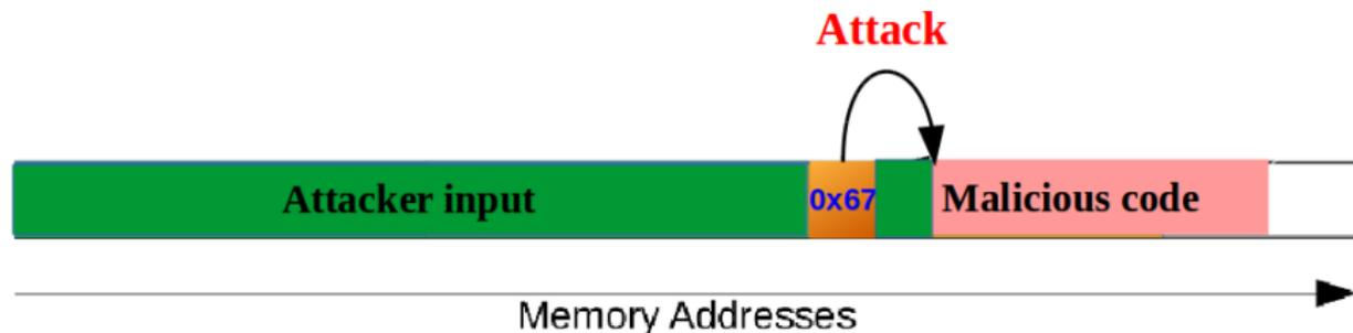
*Figure 7:* Diverting control to the injected code or existing module
